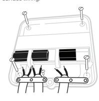
C) Replace the cover Locate the hinges at the top of the cover and wall plate, close the cover and secure with the screw.
